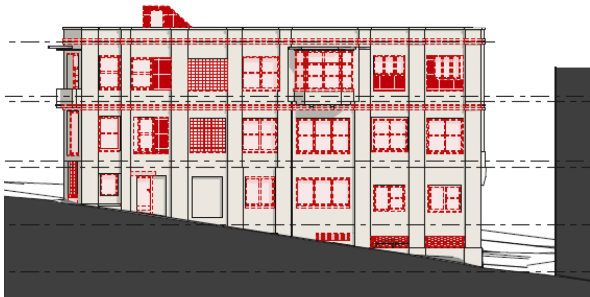
Figure 18: Proposed Langley Street elevation demolition
